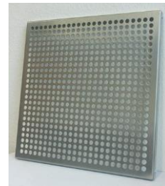
Perforation diameter 10 mm, holes in a grid spaced at 15 x 15 mm
